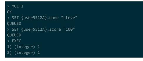
You're technically operating on 2 different keys in this transaction: {user5512A}.name and {user5512A}.score. But, because the portion of the keys wrapped in { and } are the same, they're guaranteed to hash to the same slot. As such, this transaction will work fine.
