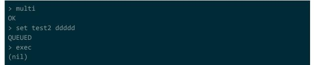
Notice the last line says "(nil)". That means that the transaction wasn't executed because the WATCH we issued detected that the value for "test1" was changed by another client.
